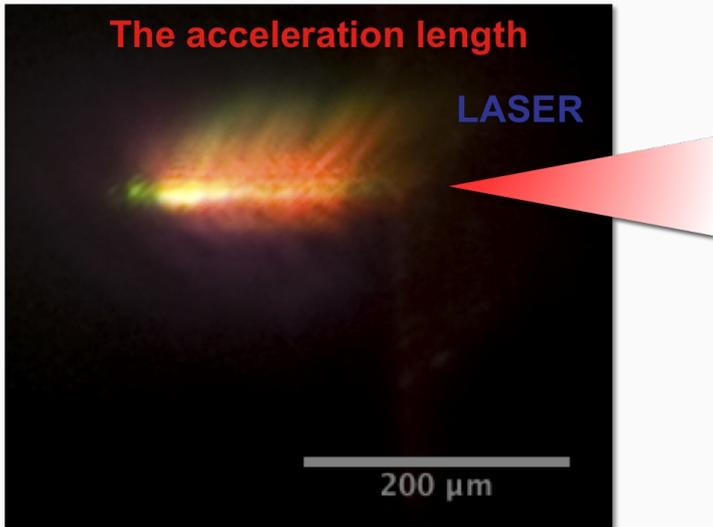
Thomson imaging clearly showed the region of propagation of the laser pulse, with evidence of self-guiding over a length approximately 2-3 times the depth of focus.
