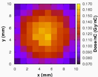
Transverse dose deposition profile uniform within  $\sim 10\%$  over a field of  $\sim 6\text{mm}$  size (appropriate for radiobiology experiments with small samples)
