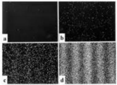
Single-electron Build-up of Interference Pattern
